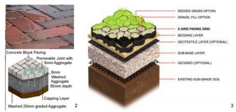
Grasscrete is a concrete structure, and not favoured for regularly used surfaces which allows grass to grow through but water to drain away through a sub base.
