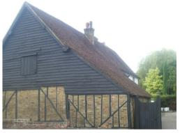
Fig 5.18 Old Mill House- timber framed barn with stained weather boarding
