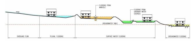
Figure 1-8 Illustration of Flood Sources (source: WSP, 2010).
