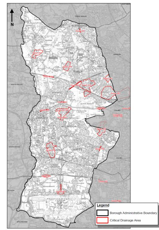
Figure i. Critical Drainage Areas within the London Borough of Hillingdon.
