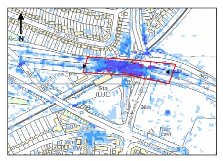
Description: Surface water is predicted to ponds in the local topographical low point located within this section of the A40 below the A437 overpass. There is no Thames Water drainage in the section of the A40 in this location and therefore it is unclear how this location drains.
